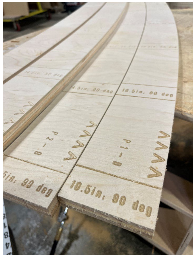
The labeling system engraves fabrication information into the CNC'd parts, including part labels, indicators for casting face side, and information on stud locations and dimensions.
