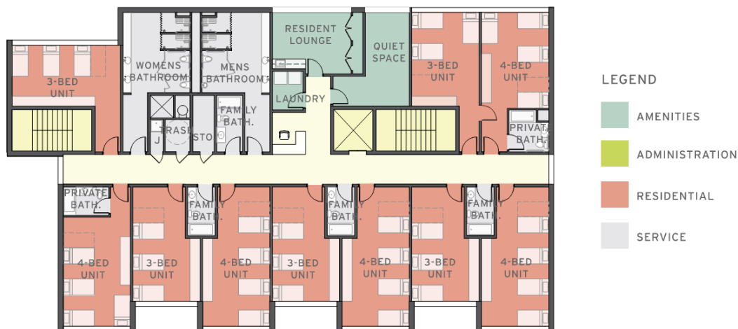
Figure 8: Case Study A layout with shared bathrooms and family bathrooms; Source: CS-A's Schematic Design Report
