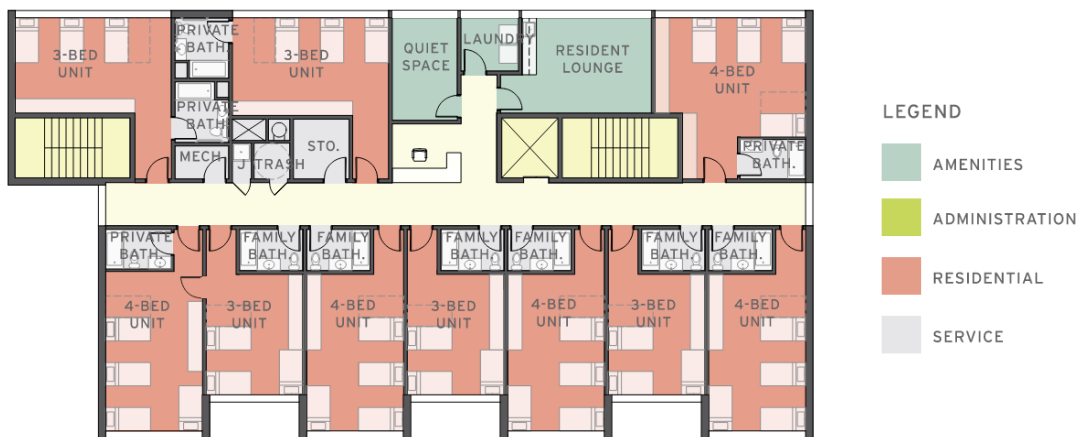
Figure 7: Case Study A layout with private en-suite bathrooms and family bathrooms; Source: CS-A's Schematic Design Report
