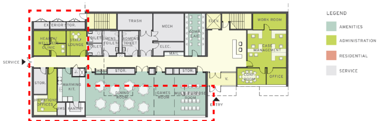
Figure 19: Initial ground floor plan with bump-out indicated; Source: CS-A Schematic Design Report
