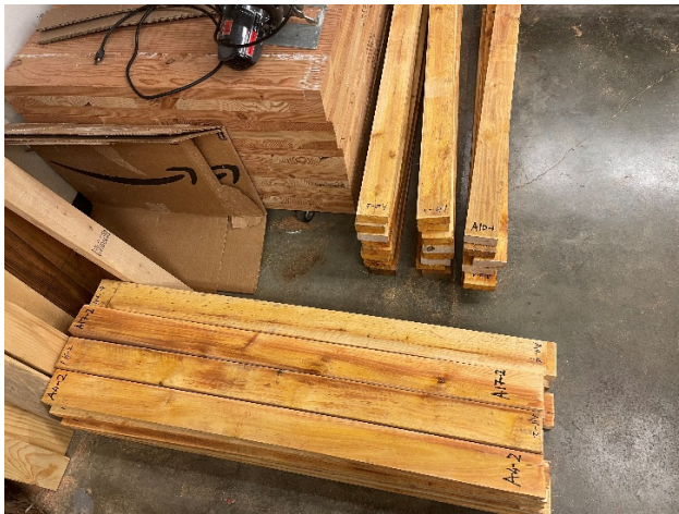
Figure 3: Two separate stacks of 24 4 ft. pieces of lumber
