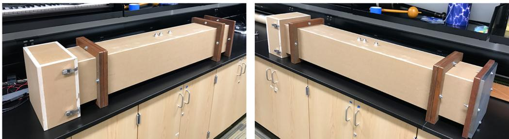
*Figure 69: View of the completed impedance tube setup*
